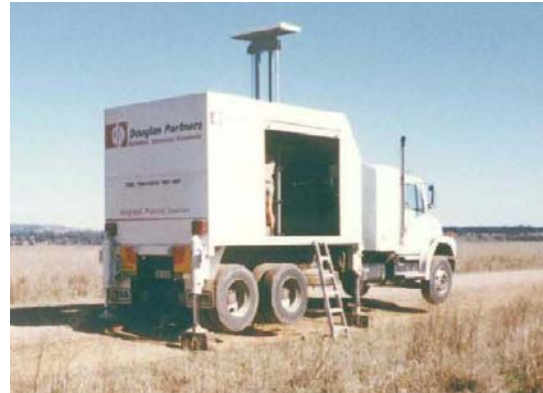
Figure 2: Purpose built CPT rig
